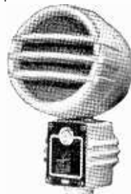
The UNICORN, model H21. A miniature exponential horn type speaker of novel design and construction (prov. patent). Ideal for noisy locations, vehicles, etc. Handling capacity approx. 5 watts, impedance 15 ohms.
